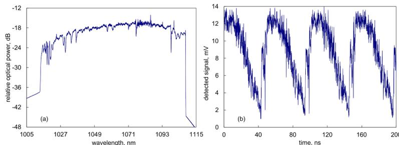
Figure 2. The measured outputs of the SPML laser. (a) The laser provides a sweeping range of over 92 nm at a center wavelength of 1060 nm. (b) The laser produces a repetition rate up to  $\sim 20$  MHz at 100% duty cycle.
