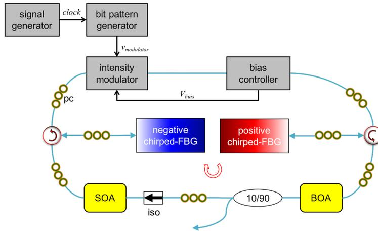
Figure 1. A schematic of the stretched-pulse mode-locked laser at 1060 nm. SOA: semiconductor optical amplifier; BOA: booster optical amplifier; iso: isolator; chirped-FBG: chirped fiber Bragg grating ( $\pm 556$  ps/nm at 1060 nm), pc: polarization control pedal.
