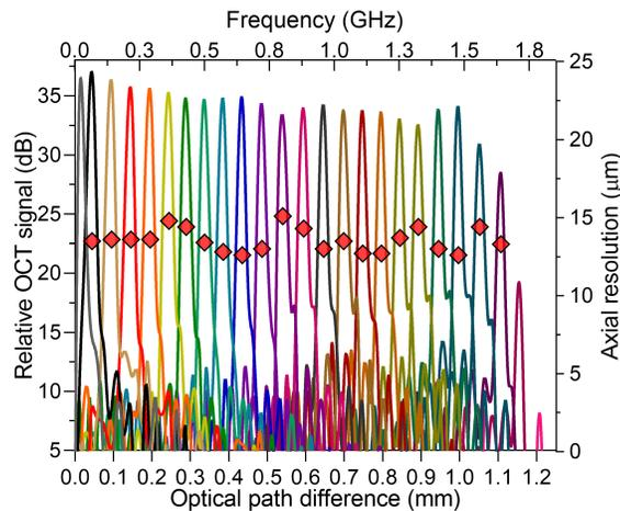
Figure 4. Point spread functions for multiple mirror distances in the air. The coherence length was  $>1.0$  mm. The axial resolution was measured to be  $12.5 \mu\text{m}$  at the mirror distance of  $0.1$  mm.
