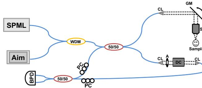
Figure 3. A schematic of the fiber based balanced Michelson interferometer. Aim: aiming beam; PC: polarization control pedal; BPD: balanced photodetector; WDM: wavelength division multiplexer; CL: collimating lens; SL: scan lens; GM: Galvo scanning mirror; A: iris, DC: dispersion compensator.
