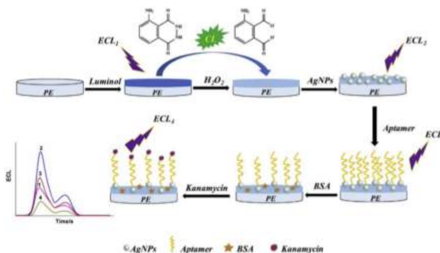
Figure 11: Schematic of the aptasensor for the detection of kanamycin (BSA: Bovine Serum Albumin). (Reprinted from [71] with permission: ©2019 Elsevier B.V. All rights reserved.).
