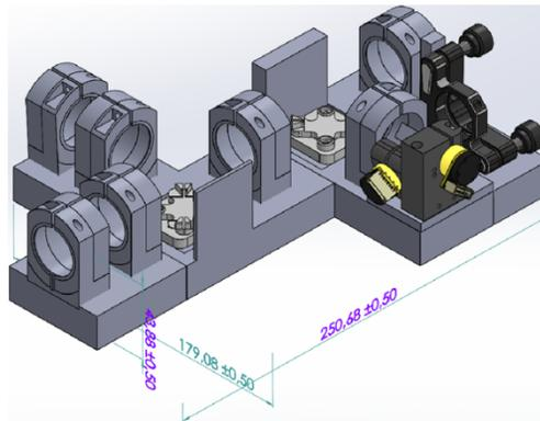
Figure 1. SolidWorks CAD drawing of 3D printable reticle head.
