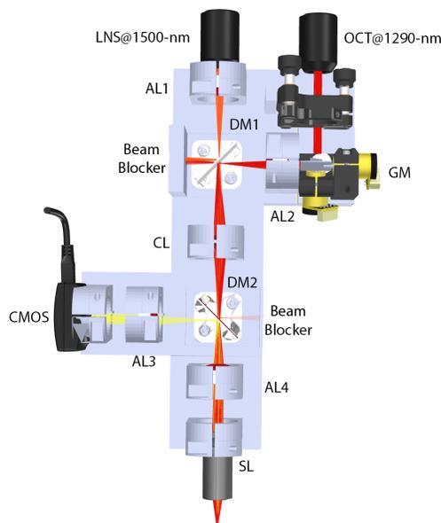
Figure 2. Ray optics simulation results. AL: achromatic lens. DM: dichromatic mirror. CL: bi-convex lens. GM: Galvo scanner. SL: scanning lens.
